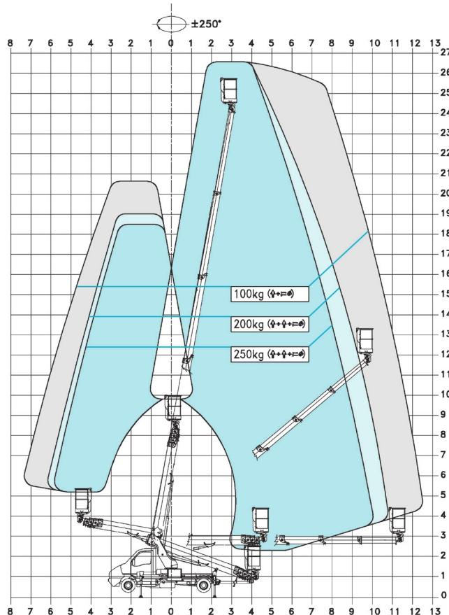
\* outreach and height max values and repeatability can change within  $\pm 3\%$  due to manufacturing variation and working condition.
